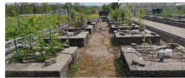
lyismeters setup under field conditions.
